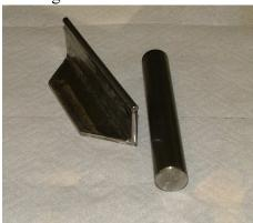
After welding the posts to the steel angle which had already been cut to size, all that remained was to epoxy the ½" rod to the top edge and paint them. I wanted a small tool rest for pen turning., a longer then standard tool rest (16") for reaching into deep bowls and a 90 degree corner tool rest.
